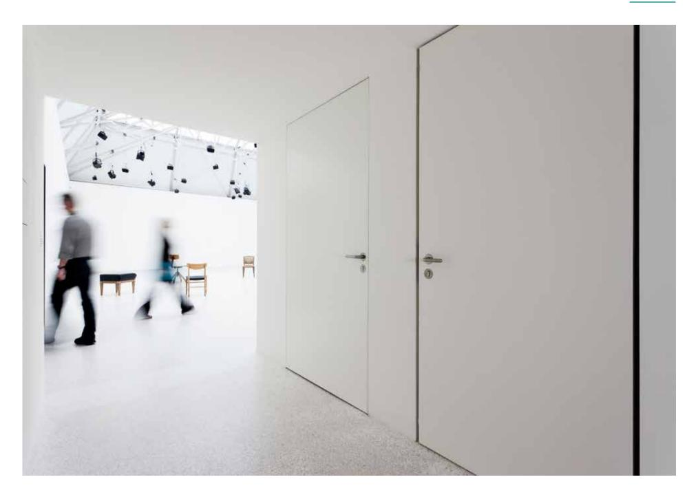
Integration of a door into a surrounding wall without a visible frame.
